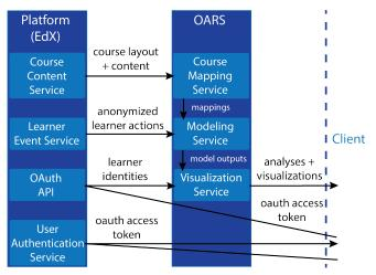
Figure 1. The OARS system is in constant communication with every linked-up learning platform, updating its analyses in real time to support immediate user inquiry. This diagram shows the data flows between OARS, the connected learning platform, and the user's browser; it also depicts the flow of data between the OARS services.
